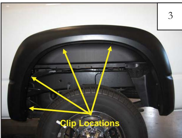
Remove flare from fender. Center a supplied black tab over each mark made in step 1.
