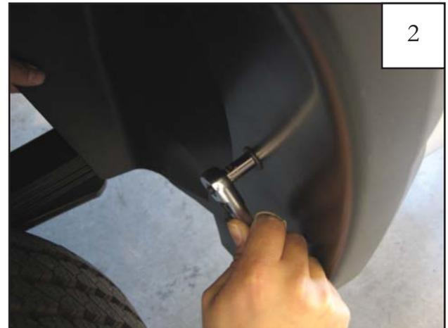
Holding flare in position on fender, reinstall screws removed in Step 1. Do not tighten. (An awl may be used to align the threaded clip with holes in flare and fender lip) Note: Make sure screws engage in splash shield.
